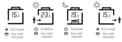
The SALUS FC600 allows you to reduce energy consumption whilst providing efficient temperature and thermal comfort in places where it is required.
