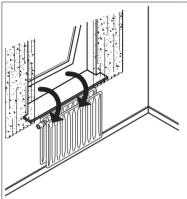
Danfoss Eco<sup>™</sup> features an Open-window function, which closes the valve if the room temperature is falling dramatically, thus reducing the heat loss.
