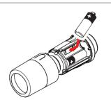
Press and hold , Keep holding while reinserting the battery. The screen will go blank after approx 3 seconds.
