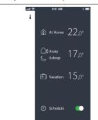
Scroll on temperatures to set your preferred temperatures. The Danfoss Eco™ can be set from 5°C to 28°C.
