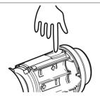
Press firmly on the tab and unscrew the thermostat from the adapter.
