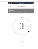
When Danfoss Eco™ is turned down to Min level manually, a notification banner is shown, and center icon switches to 'Pause'.
