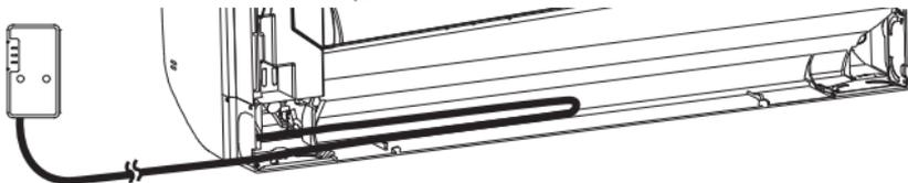
Run the connecting cable in the space on the back of the unit as shown in the above figure. Tuck cabling away and secure it.
