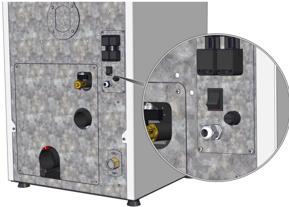
Picture 26. The positional representation of the cable grommet, main switch as well as the safety thermostat
