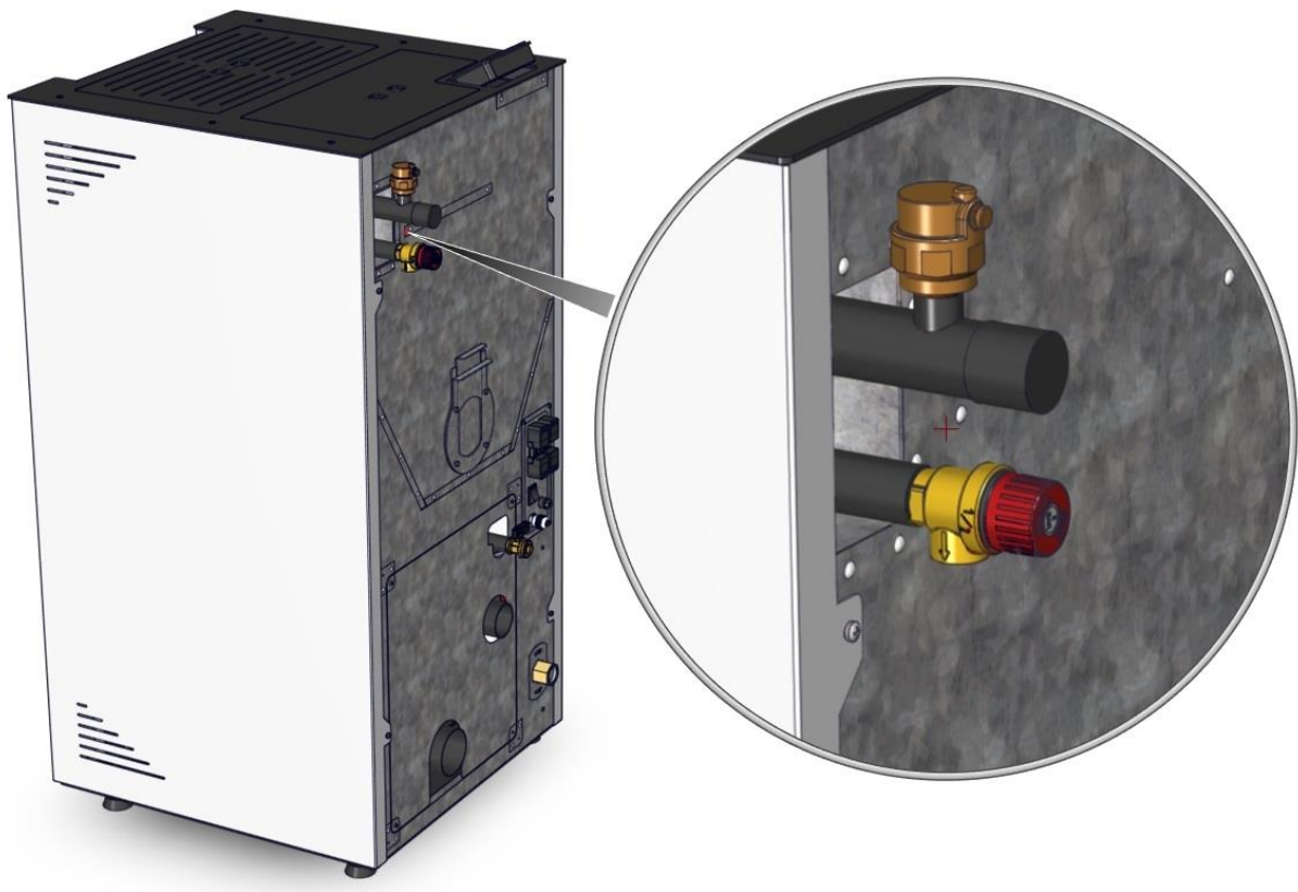
Picture 15. The representation of the air vent and safety valve at the back of the boiler
