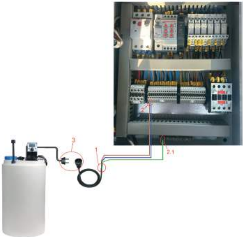
Fig. 8 – Wiring diagram for industrial reverse osmosis systems with controller OC5000 and OC6000 (constant dosing)
