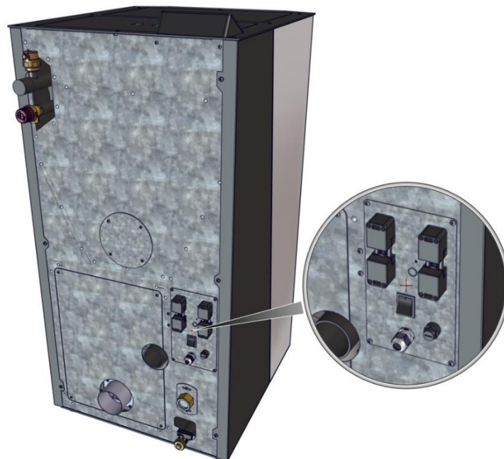
Picture 26. The positional representation of the cable grommet, main switch as well as the safety thermostat
